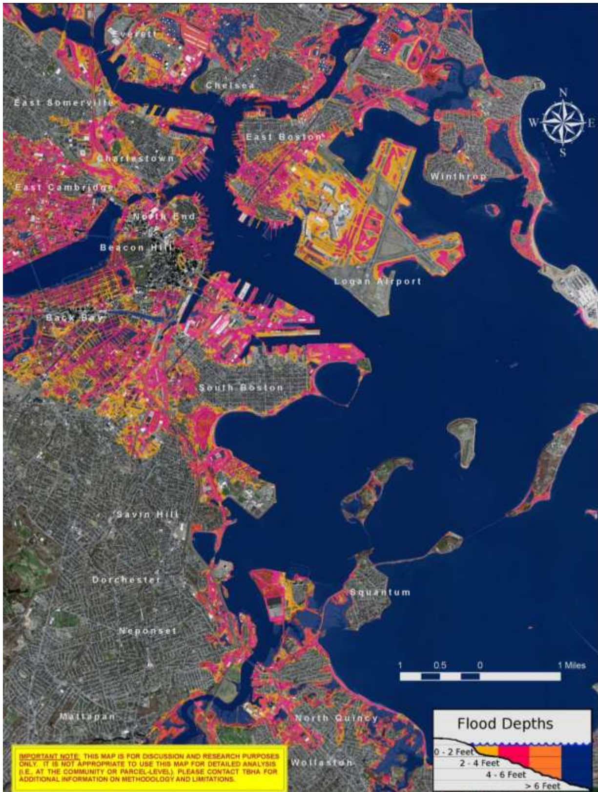
Figure 9. Plausible flooding in Boston at a sea level of MHHW+7.5/12.3 ft NAVD (TBHA, 2010).
