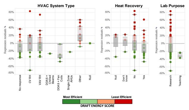
Figure 16: Residuals (Energy Score) for Bio/Biochem and Chemistry Buildings as a Function of HVAC System Type (Left), Presence of Exhaust Heat Recovery (Middle), and Lab Purpose (Right). Data Point Colors Represent Energy Rankings.
