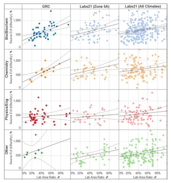
Figure 12: Source EUI by Lab Type vs. Lab Area Fraction for the GRC sample (left), the Labs21 Climate Zone 5A Sample (middle), and the Full Labs21 National Sample (right)
