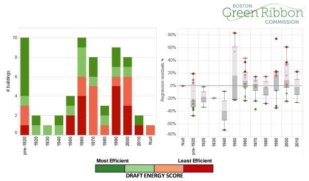
Figure 15: Energy Ranking by Decade of Construction (Note: Left and Right Figures Show Same Data). Colors of Columns and Data Points Represent Energy Rankings.
